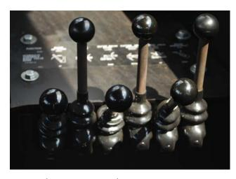
Lever-style operator controls provide precision positioning of the booms and cutter heads.
