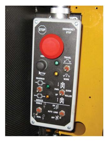
Seat-side controls allow quick switching between manual and automatic autofeed as well as single- and dual-workhead modes.
