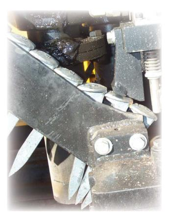
Operators control how spikes feed into the driving guns - selecting between manual or automatic mode.
