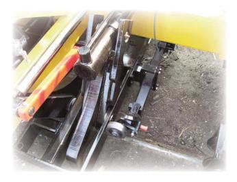
The gauger assembly allows rapid, yet extremely accurate, track setting at the correct gauge.
