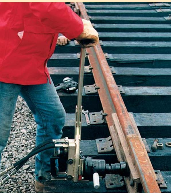
Stanley's hydraulic impact wrenches are world renowned for their adjustable impact intensity settings allowing for a wide range of uses. The rugged design incorporates an integral motor and heavy-duty mechanism for the rigors of track maintenance use. The power-to-weight ratio of these products are un-matched by any impact wrench on the market in their class.
